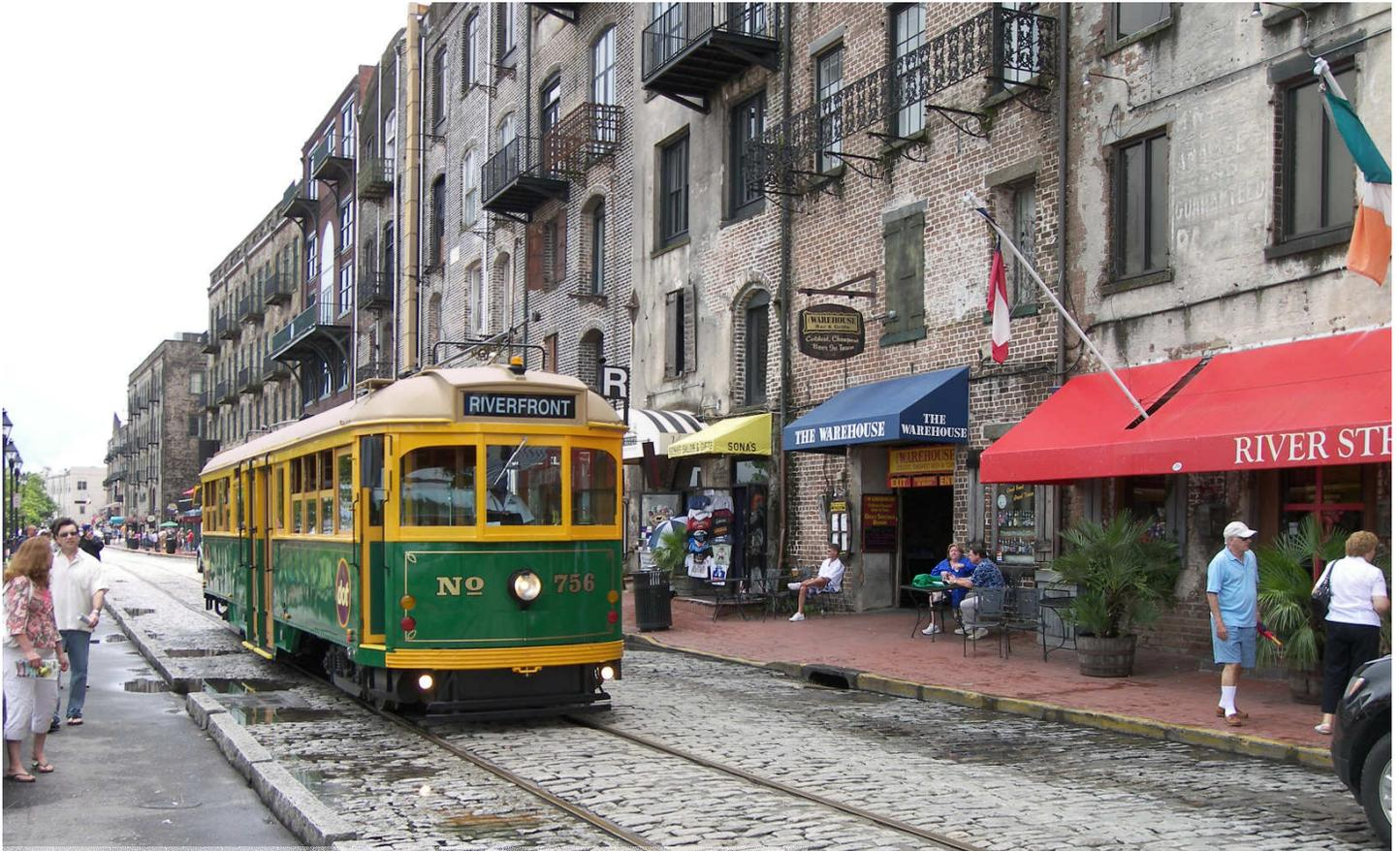
Since this past February the City of Savannah has operated a renovated 1925 W5 streetcar from Melbourne, Australia. The 47-foot car quietly burns recycled biodiesel to run on-board electric generators. The 3/4-mile River Street route is FREE, and makes five stops.
