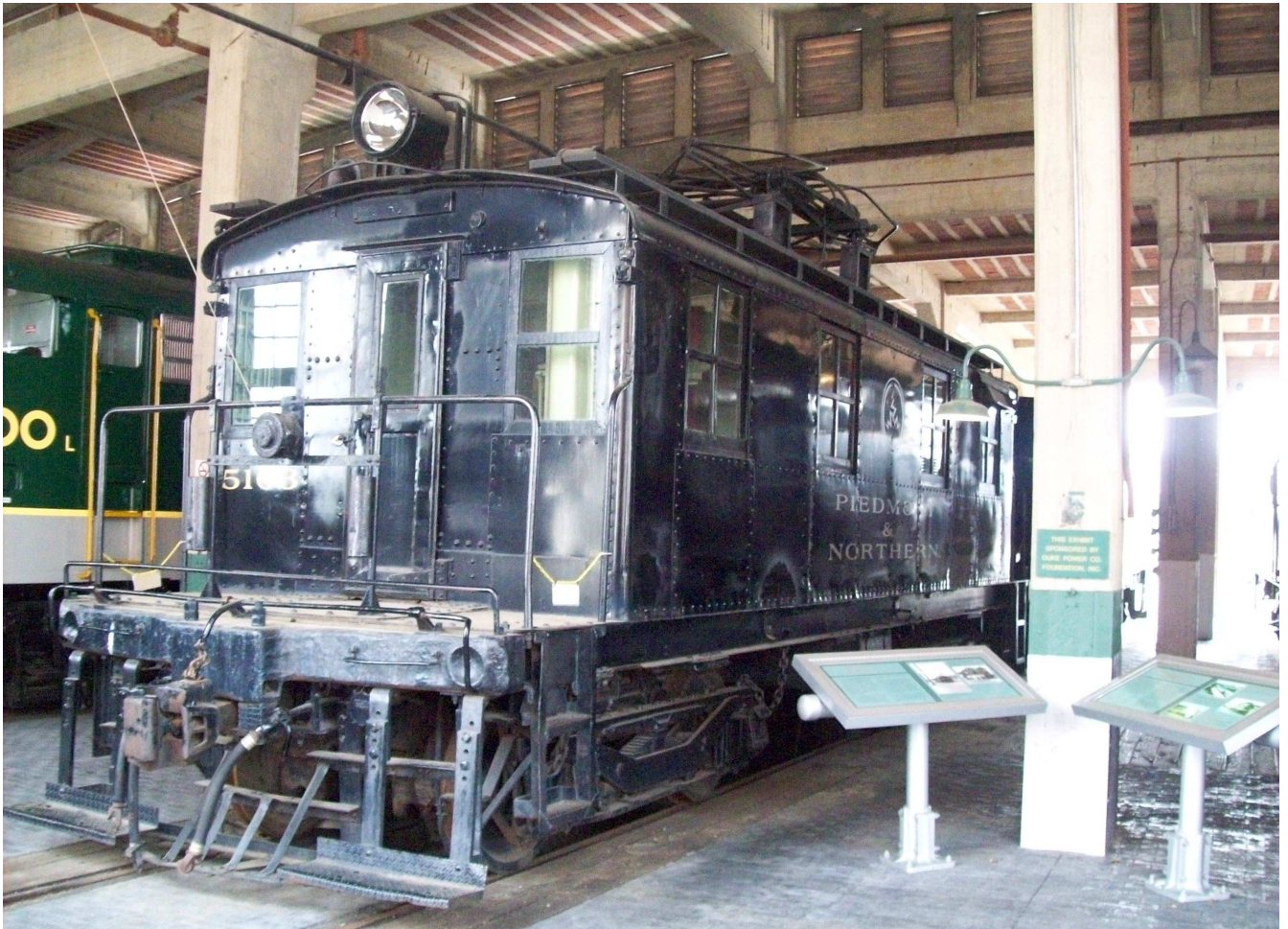
Piedmont & Northern’s GE class 404-E-120-4-GE-212F 63-ton boxcab electric locomotive #5103 on display at the North Carolina Transportation Museum at Spencer Shops, NC. Photo by J.T. Thorpe
